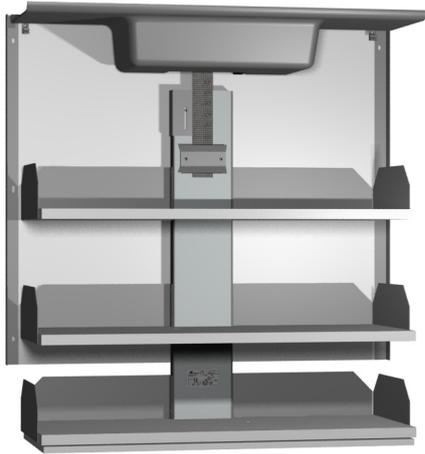
The Verti Cabinet lift unit comprises a rear panel, to be mounted on a wall, a lifting mechanism and a rack with 3 shelves. The vertical lifting and lowering motions are made by an electrically powered lifting belt, which is fitted between the rear panel and the shelf rack.
